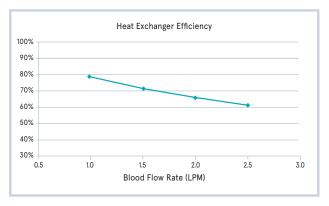
Performance data: D100 and D101 In vitro tests with bovine blood at AAMI standards conditions Hgb:  $12 \pm 0.2$  g/dl B.E.:  $0 \pm 5$  mmol/l Blood Temp.:  $37 \pm 1$  °C  $O_2$  Venous Sat.:  $65 \pm 5$  % Venous pCO $_2$ :  $45 \pm 5$  mmHg Water flow rate at water side = 10 lpm
