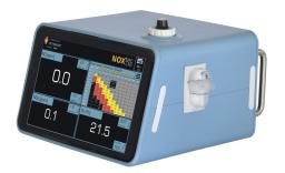
NOXtec 3000 is a medical device which monitors the supply of nitric oxide (NO), a gaseous vasodilator used to treat pulmonary arterial hypertension. Thanks to the continuous sampling of the flow supplied to the patient, NOXtec 3000 is able to determine the NO concentration that the patient is receiving, and to check if this value is placed within predetermined thresholds.
